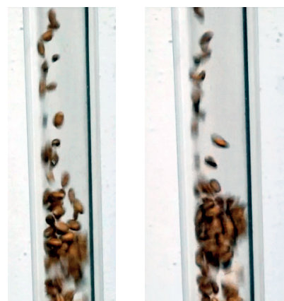
Figure 2. Flow structure during vertical pneumatic transportation of wheat grains
