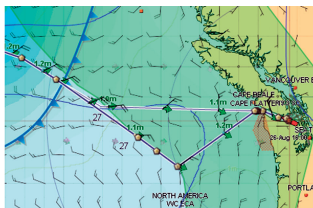
Figure 10. Route leading through the ECA Zone, optimized in the BV system (bold) and route programmed manually (Applied Weather Technologies, 2014)
