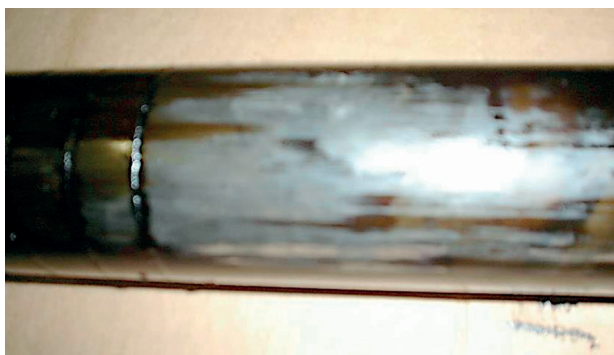
Figure 3. Traces of seizure on the fuel pump plunger, No. 1 unit after failure
