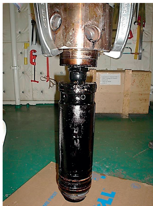
Figure 2. Dismantled barrel of fuel pump, unit No. 1 after failure
